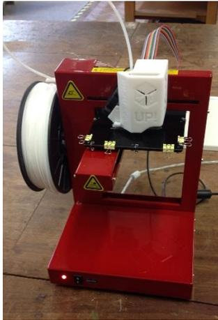
On the previous day I created the first object using Pro/DESKTOP 8. I saved the file as an STL file and loaded the file into the UP software. The software placed the object and worked out any necessary support material. The machine then printed out our first 3D object in 45 minutes.
